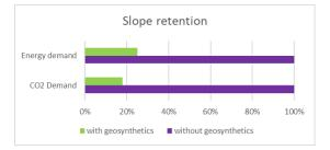
Note: Each 3 linear meters soil retaining wall (3 m high) saves 30,000 MJ-eq, which is equivalent to the energy consumption of one household per year!
