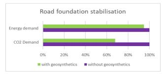
Note: When compared to lime/cement stabilization, a geosynthetic solution saves 30 % in  $CO_2$  equivalent)
