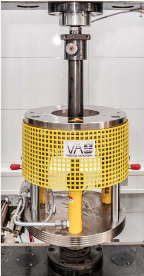
Figure 5 – EN ISO 12236 Geosynthetics – static puncture test (CBR test) - Simulation of the penetration of a stone through a geotextile for classification of the robustness class.
